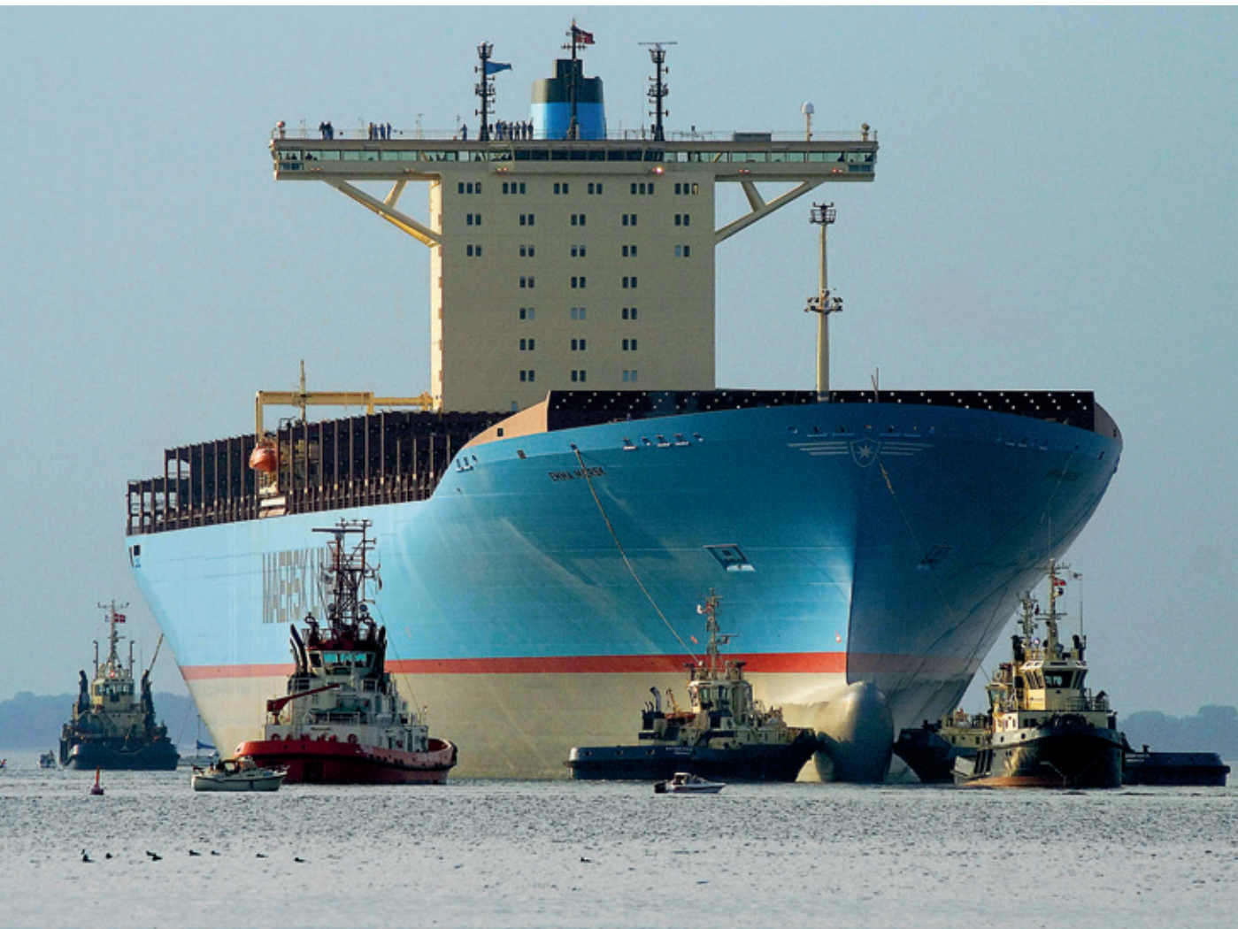
Emma Mærsk is the world's largest container vessel, measuring 397 metres long, 56 metres wide and able to carry 11.000 TEU. Photo Maersk Lines 2006.
